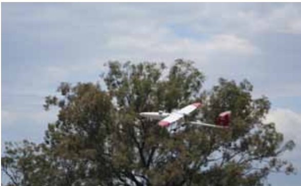
Flamingo airframe (4.1m wingspan) integrated with Micropilot™ autopilot and air sampling device
